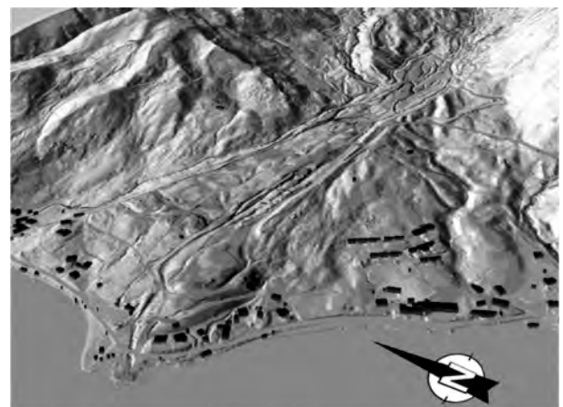
FIGURE 4: 3D view of the Gschliefgraben landslide (analytical hillshading, ALS, slant view from SW).
