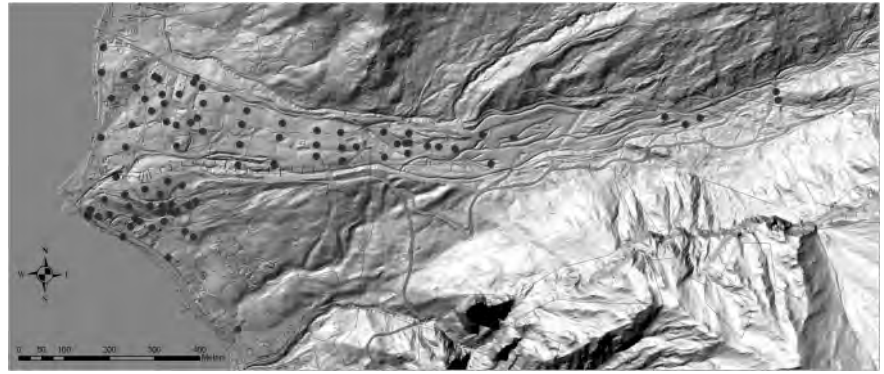
FIGURE 3: Positions of the current dGPS surveying points. Base map: analytical hillshading, ALS data.
